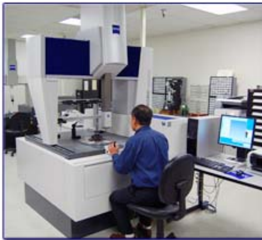
New Zeiss Prismo Navigator CMM with Rotary Table, Scanning Technology and Precise Gear Analysis System
